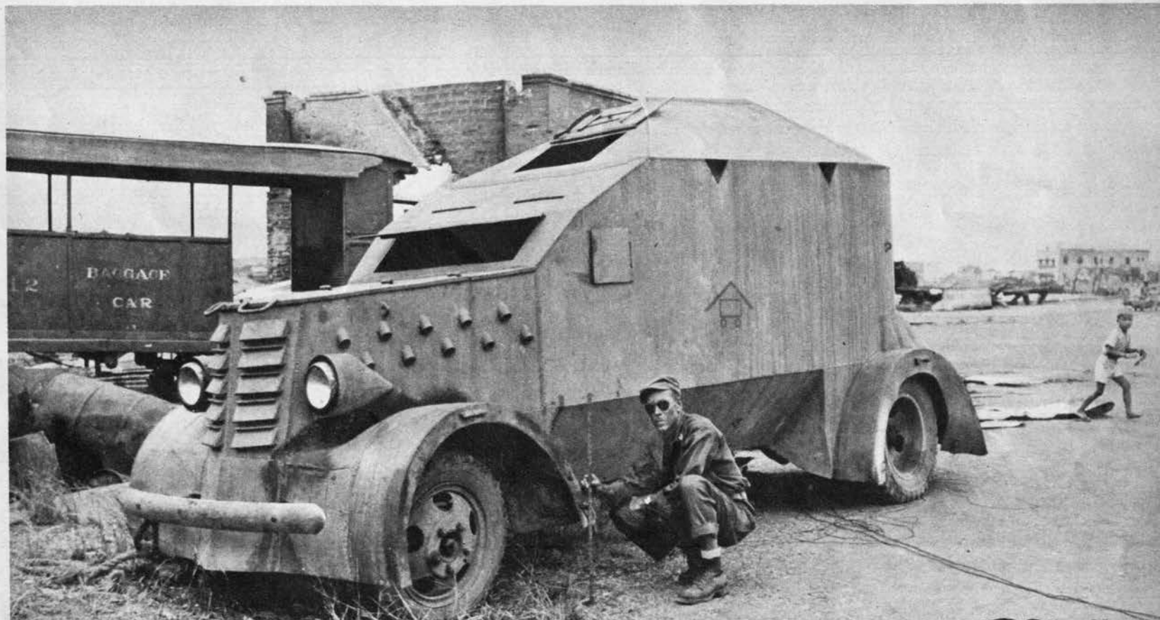
ARMORED CAR HAS BEEN CONVERTED FROM ONE-AND-A-HALF TON FORD TRUCK BY THE JAPS. IT WAS RECOVERED IN NORTHWEST PACIFIC AREA
